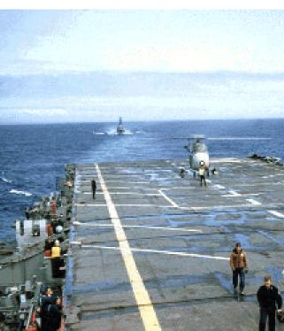
minutes. In the distance behind the aircraft carrier can be seen the plane guard destroyer. In the event that the helicopter should be unable to effect a recovery this destroyer could lower a sea boat. Since the helicopter did not fly at night the destroyer was on-call throughout all hours of darkness when fixed wing flying operations were in progress.
