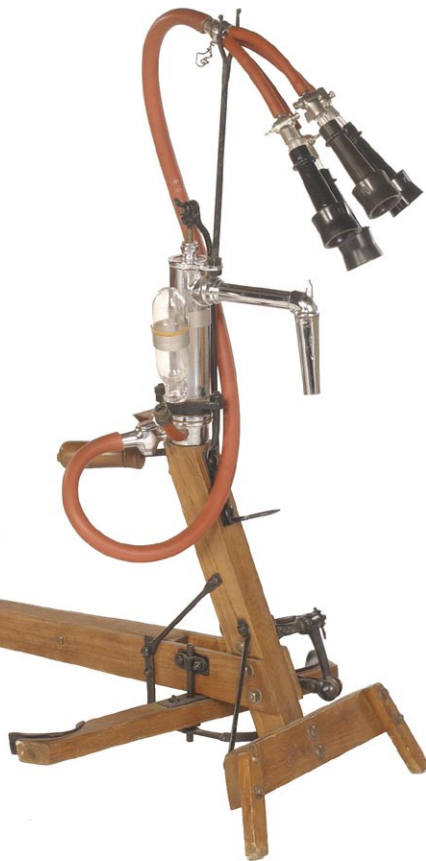
Above: The operator sat on the Wm. M. Mehring milker and “rowed” with his feet to create suction to milk the cow (780484).
