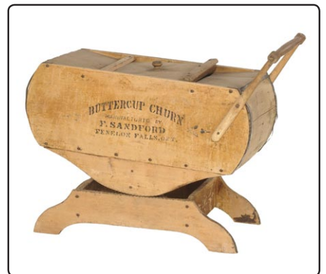
The Buttercup churn rocked on its base like a baby cradle. Baffles inside the churn agitated the cream with a figure-eight motion (840246).
