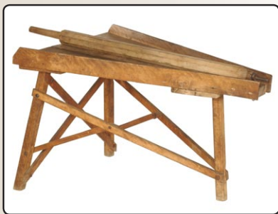
The roller’s movement forced milk out of the butter, and the liquid drained out the pointed end of the table into a waiting pail. Salt was worked through the soft butter with the same action (691148).
