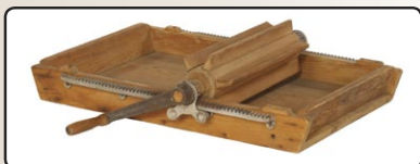
The roller in De Laval’s “Philadelphia” could be cranked back and forth over the mass of butter. De Laval was known as a supplier of everything “dairying” from farm to factory (800749).
