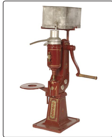
The cream separator's bowl, spouts and disks all had to be washed in hot water after each use to remove rancid milk that might contaminate the next batch (D2780 3012C).
