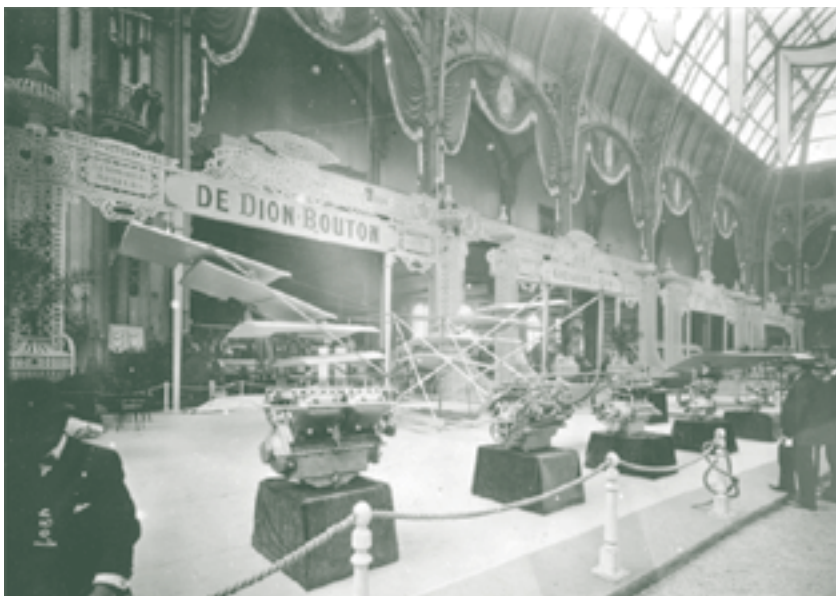
Stranger still was the de Dion-Bouton airplane with its four propellers and ten half-wings, seen here with some engines made by the Établissements de Dion-Bouton. A great automobile pioneer, the Marquess Albert de Dion (b. 1856) had co-founded the Aéro-Club de France in 1898. (1909-05-10 CAVM, Austro-Hungarian Collection, neg. no. S 23)
