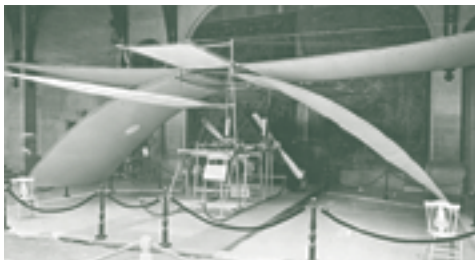
It was the hope of the Aimé-Salmson autoplane's designers that their unique-looking aircraft would be able to rise vertically into the air, fly like a conventional airplane and land, also vertically, on any small piece of ground. (1909-05-09 CAVM, Austro-Hungarian Collection, neg. no. EX 22)
