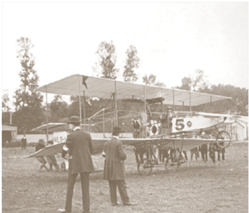
Tail-first designs proved very popular during the early days of aviation. Guillaume Busson (b. 1885), for example, flew a Witzig-Lioré-Dutilleul (WLD) biplane at the Port-Aviation air meet. This fledgling aviator may have damaged his airplane later on. (1909-06-08 CAvM, Austro-Hungarian Collection, neg. no. W 1.1b)
