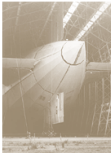
The original pointed tail of the R.100
