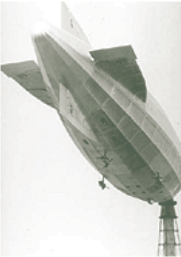
The R.100's new rounded tail
