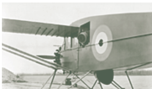
The development of aircraft, equipment and aerial photographic methods continued throughout the 1920s and 1930s. Shown is a multi-camera installation in an RCAF Bellanca Pacemaker, Rockcliffe, 1935. (Public Archives of Canada PA 63075)
