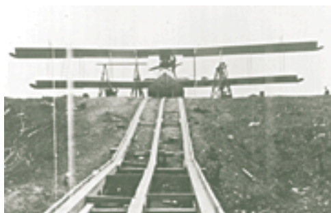
An Air Board Curtiss HS-2L at the top of the primitive slipway at Rockcliffe in 1922. In 1925, the Ottawa Air Station was moved 24 km up the Ottawa River to Shirley's Bay because the high river banks at Rockcliffe made the beaching of seaplanes and flying boats a major problem. (Department of National Defence RE 18032)
