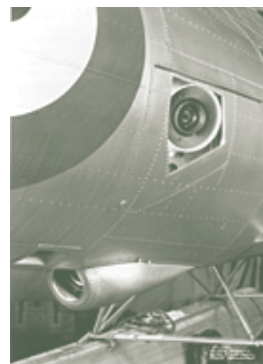
Exterior view of multi-camera installation in a Fairchild Super 71, Rockcliffe, 1936. (Public Archives of Canada PA 63180)
