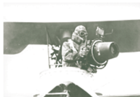
Since its earliest days as an airfield, aerial photography had been conducted from Rockcliffe. Here an observer operates the oblique aerial camera mounted in a Vickers Vedette flying boat, 1931. (Public Archives of Canada PA 62895)
