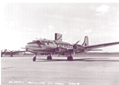
The 1950 version of the “Rockcliffe Ice Wagon” was this modified Canadair North Star. (Public Archives of Canada PA 66191)
