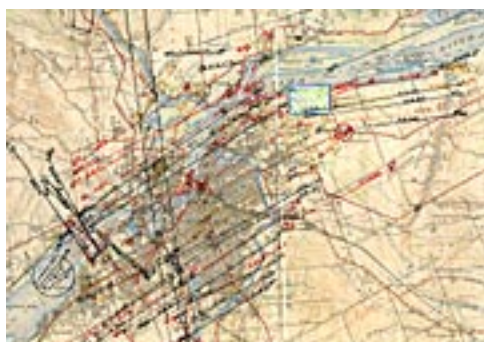
This reference map shows the flight lines followed for the aerial plotting of photographs taken during an aerial survey of Ottawa in 1928-29. Photographs were taken in sequence along each line. For example, the photograph A190.11 was taken from a Vickers Vedette and was the eleventh photo taken along line A190. (Courtesy National Air Photo Library, Ottawa)
