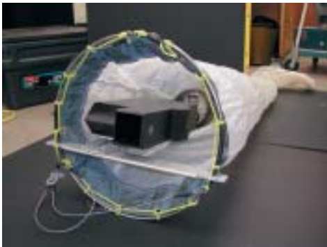
Fig. 3 The Laser-Optical Plankton Counter (LOPC) shown mounted inside a standard plankton ring net used for vertical profiling. The LOPC is capable of counting and sizing zooplankton in a range of 100 microns to 3.5 cm and can provide shape profiles of zooplankton greater than 1500 microns.
