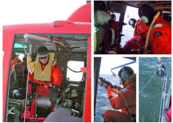
Fig. 4 Sampling using a winch powered by a cordless drill from the helicopter: the left-hand panel shows the helicopter on the ice with the CTD sampling through a hole. In-flight sampling (all other panels) is done in a similar fashion except that a second person observes the descent and gives the pilot directions to stay on-station.
