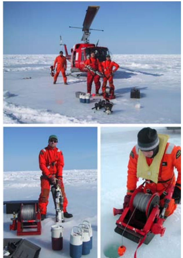
Fig. 2 On-ice station: a hole is drilled through the ice and the CTD probe is lowered to the bottom. Water samples can also be collected for later nutrient and phytoplankton analyses.
