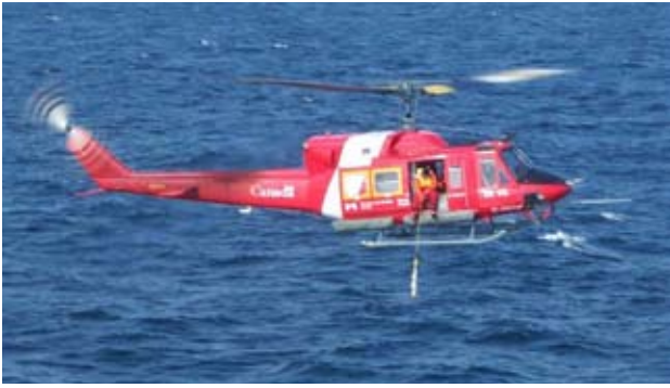
Fig. 3 Hand-powered in-flight sampling: the CTD probe is lowered into the water, 25 m below, where it is held close to the surface for one minute and then lowered to a depth of 100 to 115 m. It is then pulled back up by hand over a small pulley.
