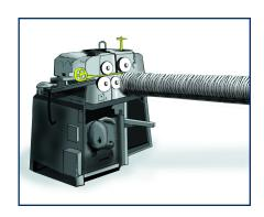
A New Brunswick worker died when his clothing became entangled in a shaft he was turning on a lathe. The WHSCC investigation revealed that the lathe was an older model that had been modified over the years and did not have the safety features of more modern lathes.
