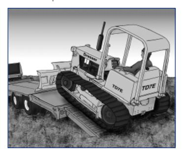
The operator was trying to load the dozer onto a tilt-up float. When the dozer reached the top of the ramps, its tracks started to spin on the float platform – causing the dozer to shift. The right track slipped off the side of the ramp and the dozer tipped over. The operator fell out of the cab and was crushed by the dozer, as it rolled onto its side.
