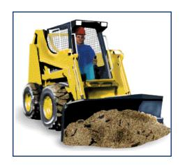
A skid steer loader is a small,quick-moving and powerful rubber tired machine — making it a versatile and potentially dangerous piece of equipment. Recently, a worker inadvertently hit the foot pedals while boarding such a loader. The bucket was activated and pinned him against the roof's edge of the cab. The accident could have been fatal.
