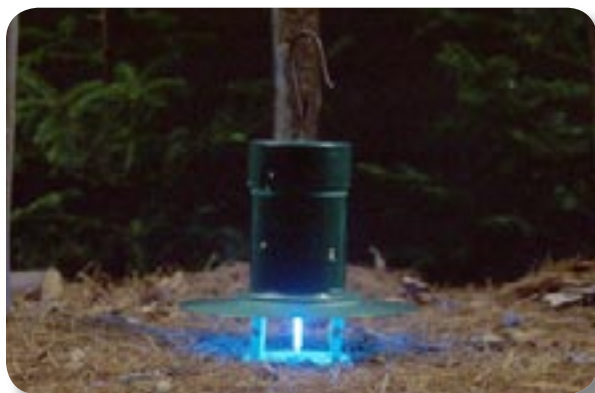
Figure 5. The Luminoc® used as a pitfall trap to collect soil-inhabiting insects.
