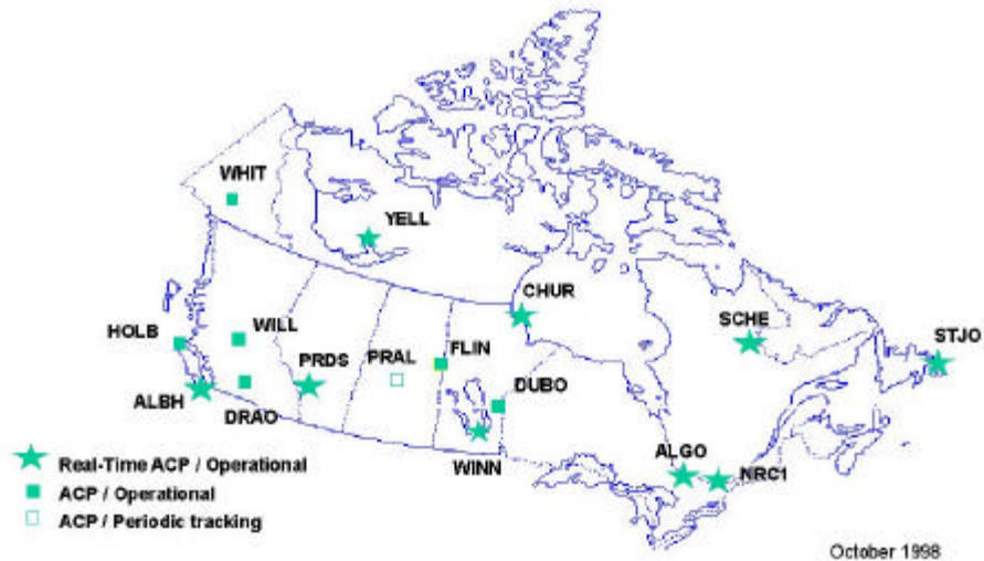
Figure 2: Network of automated stations supporting the Canadian Active Control System (CACS) [4]
