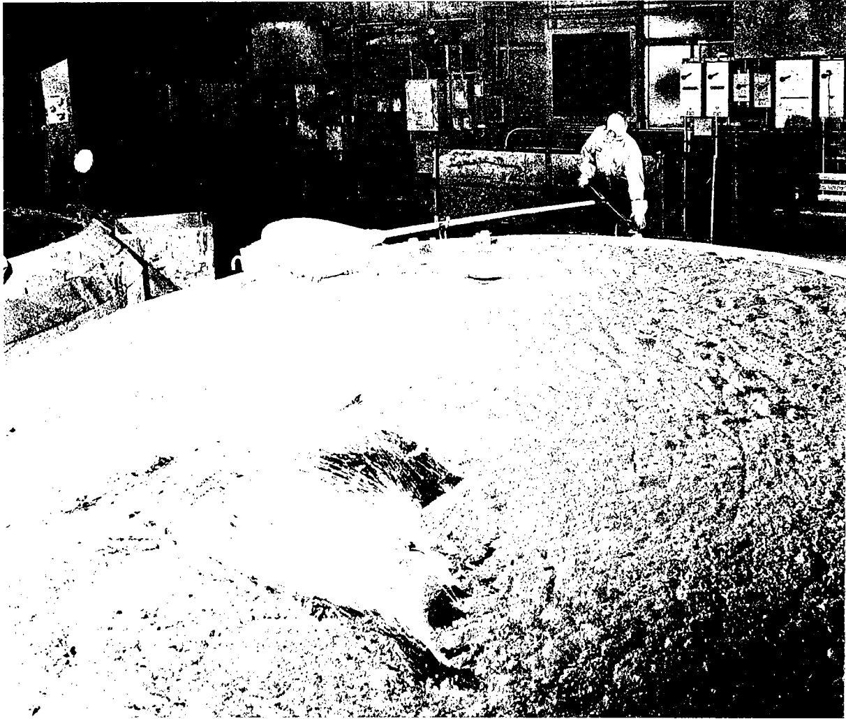
Skimming the dross from a pot of molten lead prior to casting lead pigs (ingots) at Cominco Ltd., Trail, B.C. (Cominco photo).
