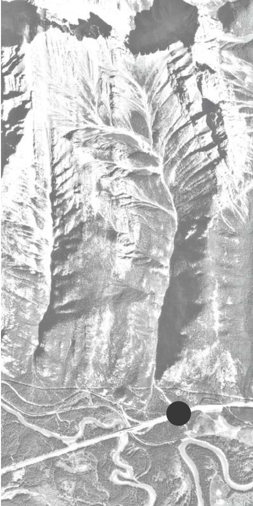
Fig. 3: Aerial photograph flown in September 1999 of % Mile Creek basin, Rocky Mountains, Banff National Park, Alberta. Bow River valley is visible in lower part of the photograph. The August 1999 debris flow originated in multiple locations within the upper part of the drainage and traveled down the creek bed to block the Trans-Canada Highway running right to left. Blockage location is denoted by black spot. The debris flow is thought to have been triggered by a very localized microburst rainfall in the upper reaches of the watershed. The debris flow blocked the Trans-Canada Highway for several days at the height of the tourist season. Aerial photographs flown specially for this project by Foto-Flight, Calgary, Alberta.
