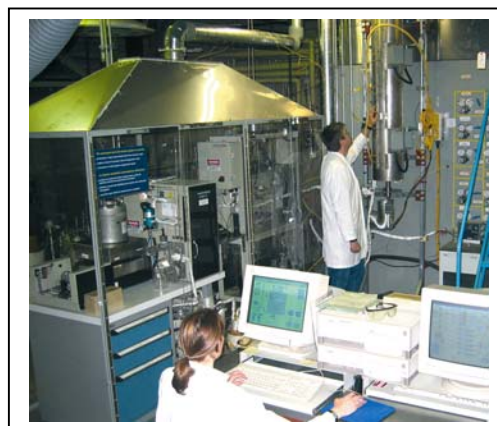
Automated reactor system used for producing cetane enhancer (SuperCetane)
