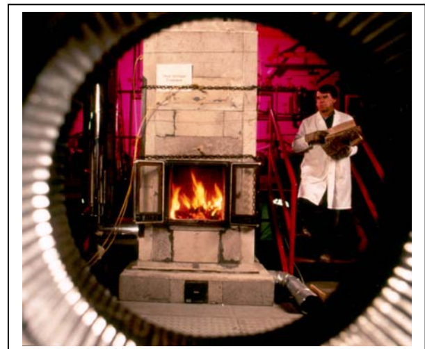
Wood Burning Fireplace under Test
