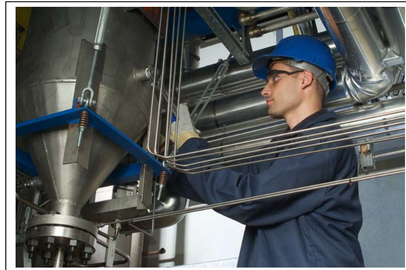
Image above: Slag is separated from the syngas in the quench vessel.
