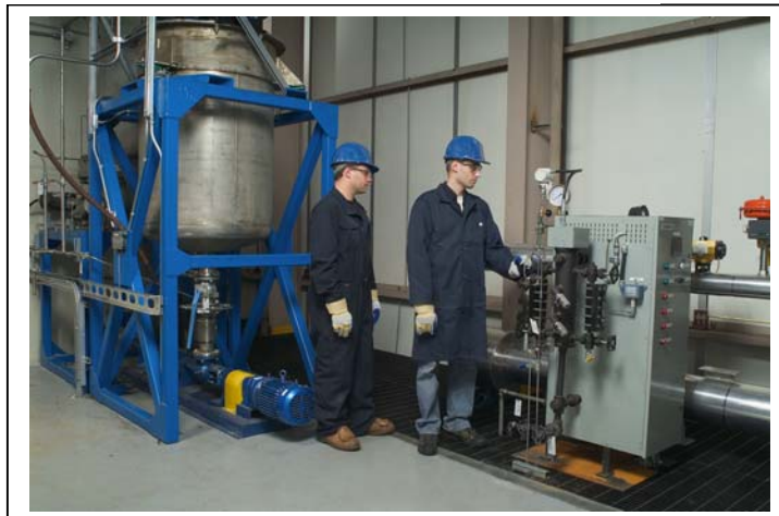
Image below: The gasifier is capable of running with a dry feed or a slurry feed.
