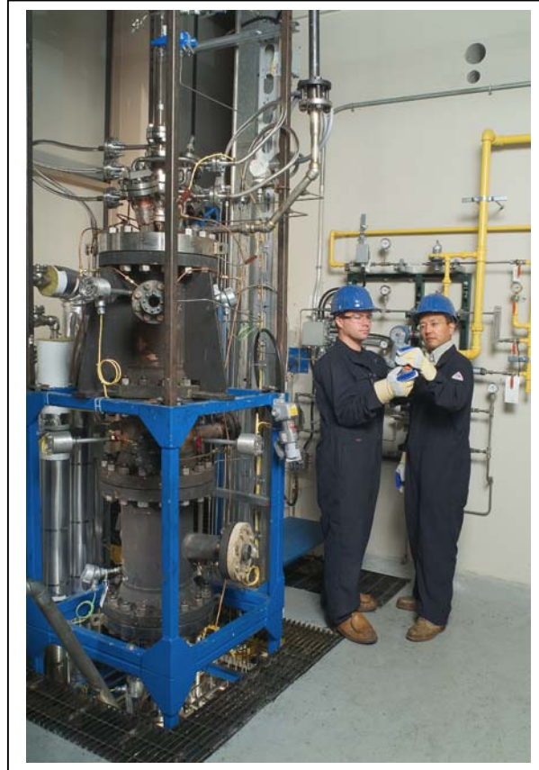
Image above: The CETC-Ottawa gasifier is sectional in design allowing modification to meet client needs.
