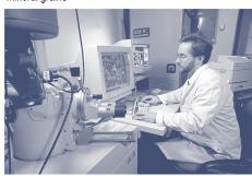
Programming an automated sample preparation machine to produce polished sections of mineral grains
