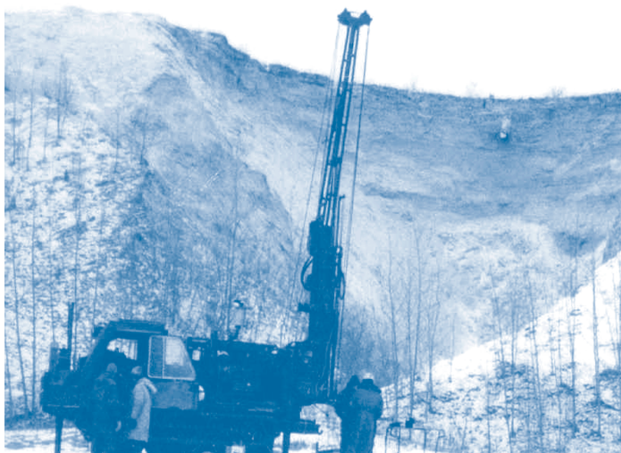
Tailings dam with progressive failure — workers conducting tests for research of material properties.
