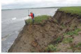
Surveying a Tundra Cliff Edge with the RTK Rover (Tuktoyaktuk Island, Northwest Territories)
