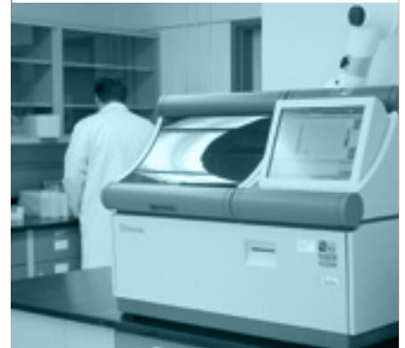
New outdoor blasting tank; X-ray fluorescence (XRF) spectrometer
