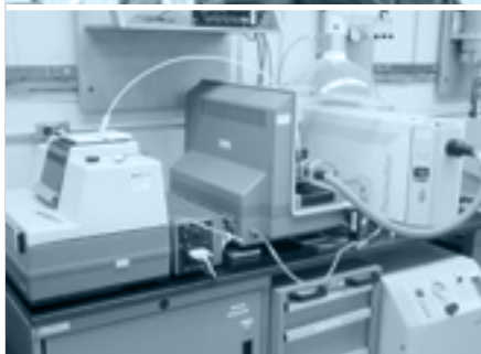
Photos from top to bottom: 1 and 2 – Assembly of a large slip ring for testing; 3 – Simultaneous TG-DTA with gas analysis by mass spectrometry and Fourier transform infrared spectrometry
