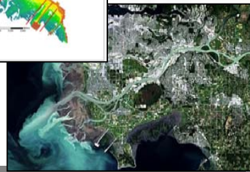
Figure 2. Satellite photo of Fraser River Delta and surface elevation map of Roberts Bank. Wave and tidal current monitoring and modeling will be completed along the four transects marked in red.
