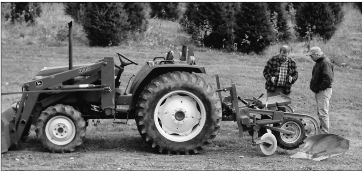
Figure 2. Mould board plough attachment with 37 hp 4X4 tractor (Photo: NRCan, AFC)
