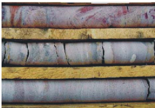
Figure 3 - Starved sequence below the MF–LzL boundary (middle row) at 365–366 m in DDH SHE-06. Note the rounded mud clasts. Core is 40 cm wide and way up is to the right.
