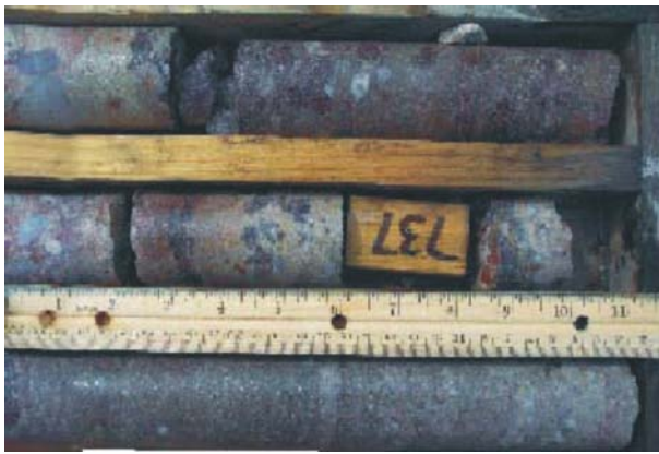
Figure 6 - Cross-bedded sandstone and conglomerate of Facies Association 1 ("Shea Creek" or Fair Point sequence at 737 m in DDH SHE-22. Core is 30 cm wide and way up is the right.
