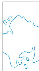
Cover features plotted with SUBCOVER command are clipped at the limits of the legend box
