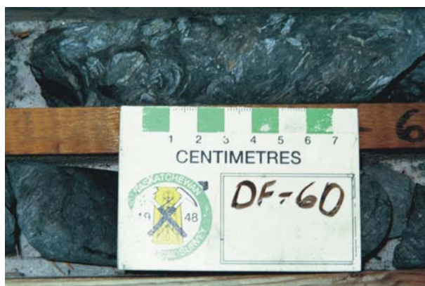
Figure 9 - Fault breccia developed in graphitic pelites along the Dufferin Lake fault.
