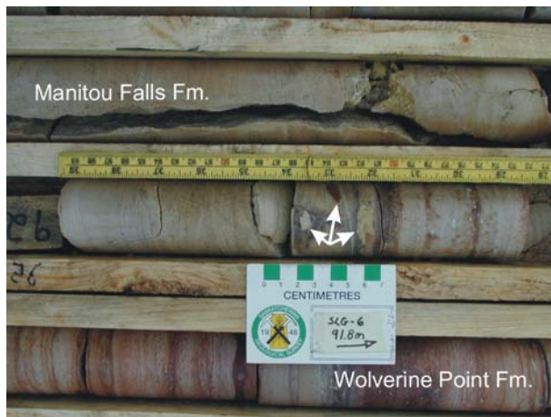
Figure 3 - Subangular to rounded, very fine-grained sandstone clasts (arrows) in a pebble lag at the base of the Wolverine Point Formation in DDH SLG-6 indicate that the contact is an erosion surface. The pebbles are associated with smaller quartz pebbles and granules in a medium to coarse sandstone matrix. Another sandstone pebble lies about a metre above the contact. Note the faulted tectonic breccia in the Mfd' at left side of the photo.
