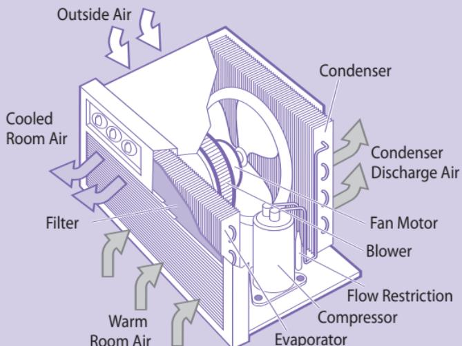
Two types of refrigerant – chlorofluorocarbons (CFCs) and hydrochlorofluorocarbons (HCFCs), such as R-22 – are being phased out under the Montreal Protocol to reduce the use and release of ozone-depleting substances. Manufacturers of all new air conditioners sold in Canada and the United States must rely on refrigerants that meet increasingly strict environmental standards. In almost all cases, older room air conditioners can't be refilled with newer refrigerants.
