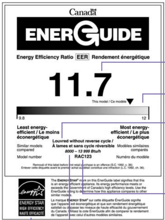
This EnerGuide label lists an EER of 11.7. Note the arrow on the scale. Its position near the far right indicates that this model is among the most energy efficient on the market.
