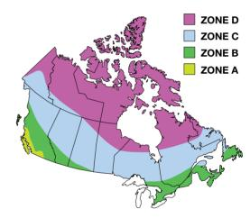
**ENERGY STAR Requirements for Windows and Doors**Products may comply based on either their U-value or their Energy Rating (ER). Windows and sliding glass doors must also have an air leakage rate of  $\leq 1.65$  (m<sup>3</sup>/h)/m.
