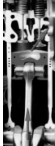
The piston on the upward stroke emits the exhaust gases.
