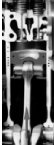
Air is heated by compression.
