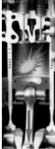
Air-Fuel mixture is ignited.
