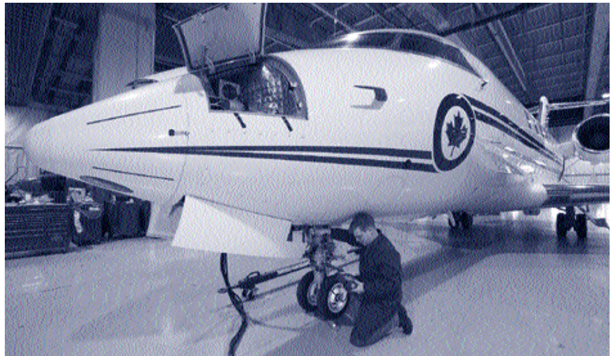
A non-destructive testing technician conducts an ultrasonic inspection to check for cracking around bolt holes in the landing gear of this CC144 Challenger aircraft. The same testing can be performed on various parts and components of the aircraft.
