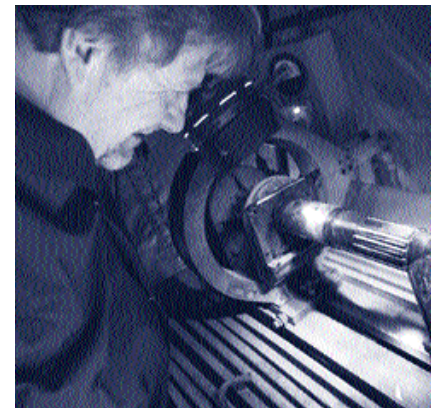
Performing a magnetic particle inspection (MPI) on an aircraft engine spline shaft. MPI is a fast and economical way to detect surface and slightly sub-surface discontinuities in ferromagnetic materials that may render the part unserviceable.
