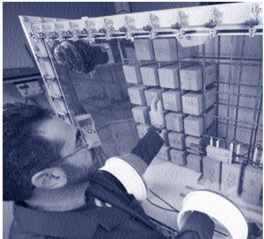
In this accelerated carbonation test machine, concrete prisms are exposed to 65% humidity and 3% CO 2 at 23°C to accelerate the diffusion of CO 2 into the concrete. At various time intervals, a slice of concrete is sawn from the concrete prisms and sprayed with a phenolphthalein indicator. The uncoloured zone identifies the carbonation depth.
