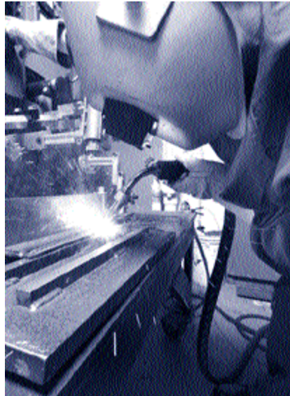
A CANMET-MTL welding technician performing an experimental MIG (metal inert gas) welding trial to establish optimum welding conditions for the production of lap welds for advanced high-strength steels.
