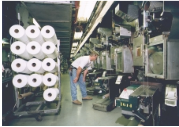
Spinning Technician Gord Blenderman verifies the operation of a high-speed winder in a nylon-yarn spinning operation at the Kingston site.
