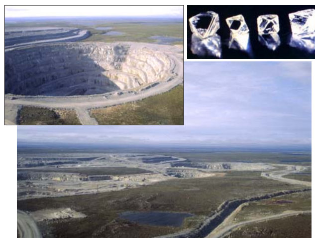
FIG. 6: North America's first diamond producer, the Ekati Mine of the central Slave craton. Main picture shows the flat barren lands of the central Slave craton, with several pipe-like kimberlite bodies being excavated in circular open pits. Inset (upper left) shows a close-up of one of the partially excavated pipes. Several mm-size gem quality diamond octahedra are shown on upper right (photos provided by David Snyder and Grant Lockhart).
