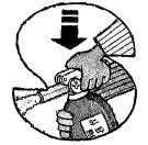
**S** — Squeeze the lever above the handle to discharge the extinguishing agent. To stop the discharge, release the lever. (Some models may have a button instead of a lever.)
