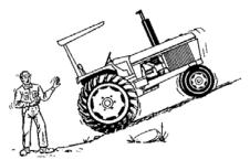
The hitch on the tractor has been designed to allow you to pull heavy loads without the risk of a backward upset. When the hitch point on a tractor is raised, the chance for a backward upset is greatly increased. Always hitch to the drawbar and keep it as low as possible.
