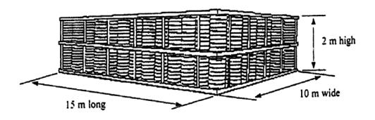
A tire storage pile of these dimensions is  $300 \text{ m}^3$  (these are sample measurements). Article 3.1 applies to volumes greater than illustrated.
