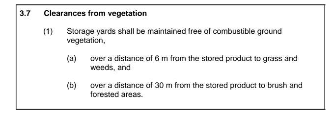
The purpose of this Article is to prevent a fire spreading along ground vegetation and involving the stored product.
