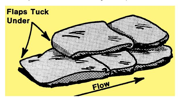
Fold the open end of the unfilled portion of the bag to form a triangle. If tied bags are used, flatten or flare the tied end.
