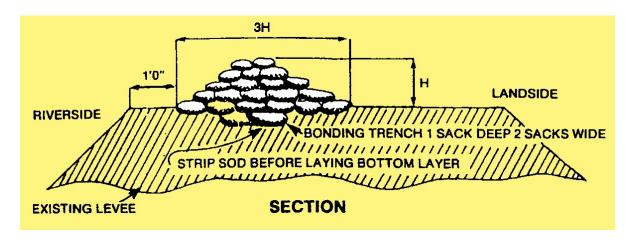
Stamp each bag in place, overlap sacks, maintain staggered joint placement, and tuck in any loose ends.
