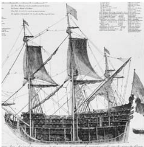
Cross-section of a 104-gun flagship giving the main dimensions and the names of the interior compartments, from Le Neptune français ou Atlas nouveau des cartes marines , by Pène, Cassini et al., 1693. FR BNF Ge CC 1114, 1 ère partie, p. 7
