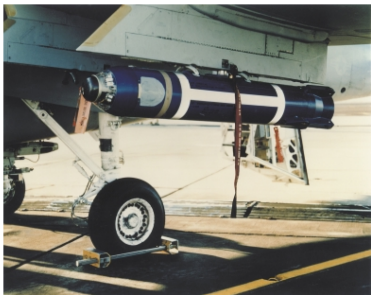
A prototype of the Big Eye (BLU-80) binary chemical bomb developed by the United States. Both binary chemical munitions and their components are defined as chemical weapons under the CWC.
