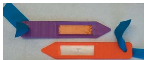
Photo 9: PRS probes, approximately 15cm long (orange - anion, purple - cation)
