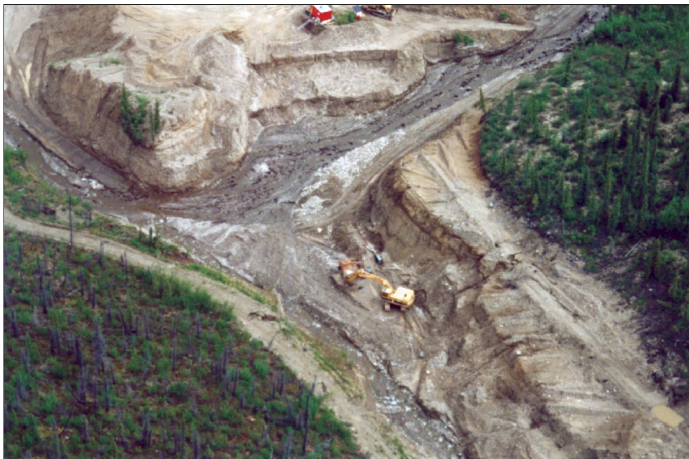
Figure 50. Aerial view of Dan Klippert's mining operation on Seattle Creek in 1997. Gold-bearing gravel was found here beneath a McConnell-age periglacial fan.
