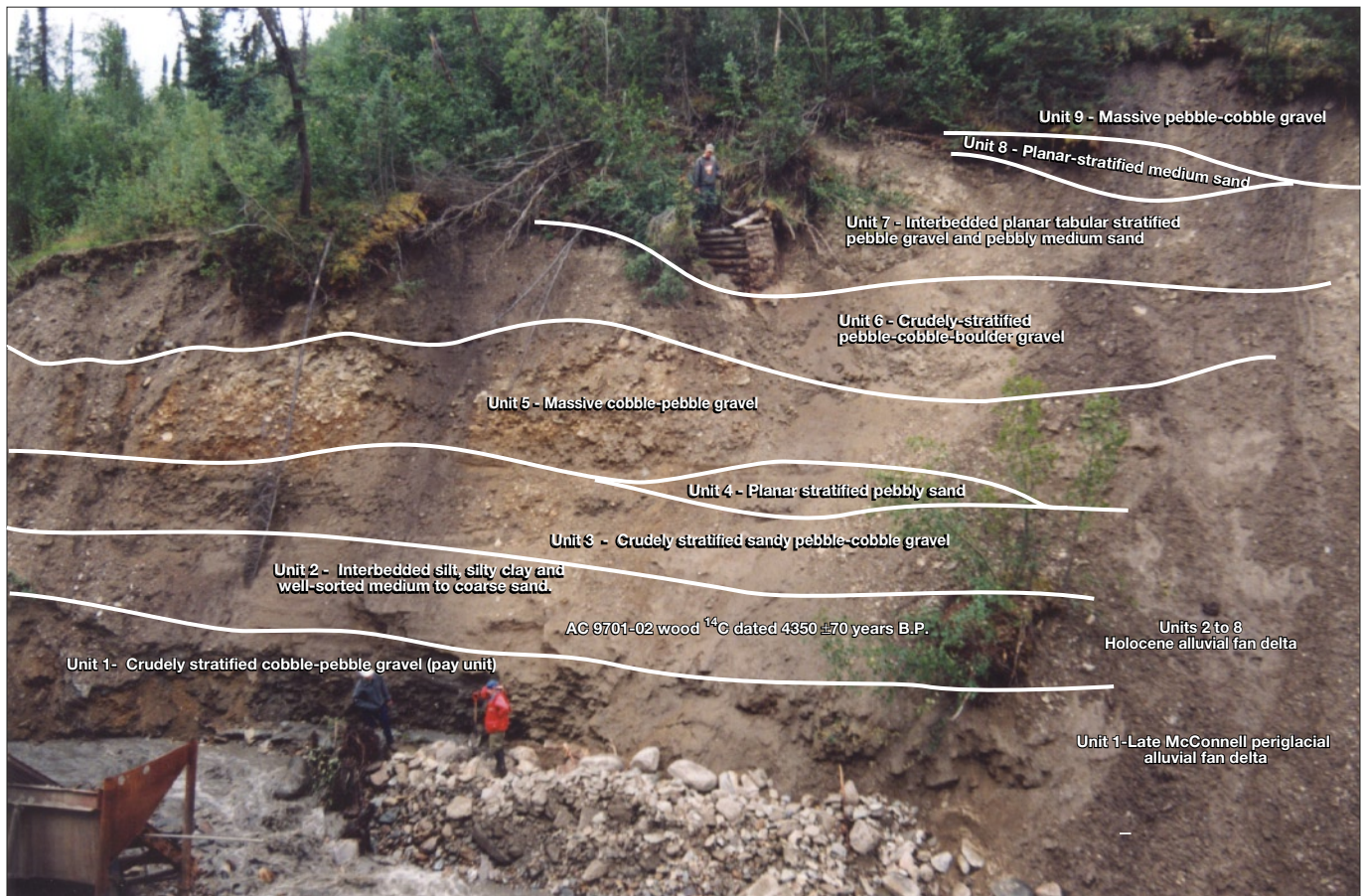
Figure 32. Panel diagram of Anderson Creek mining section showing typical alluvial fan delta stratigraphy. Alternating units of fluvial channel gravel, overbank organic silt and sand, fine-grained lake sediments and deltaic sands are characteristic.
