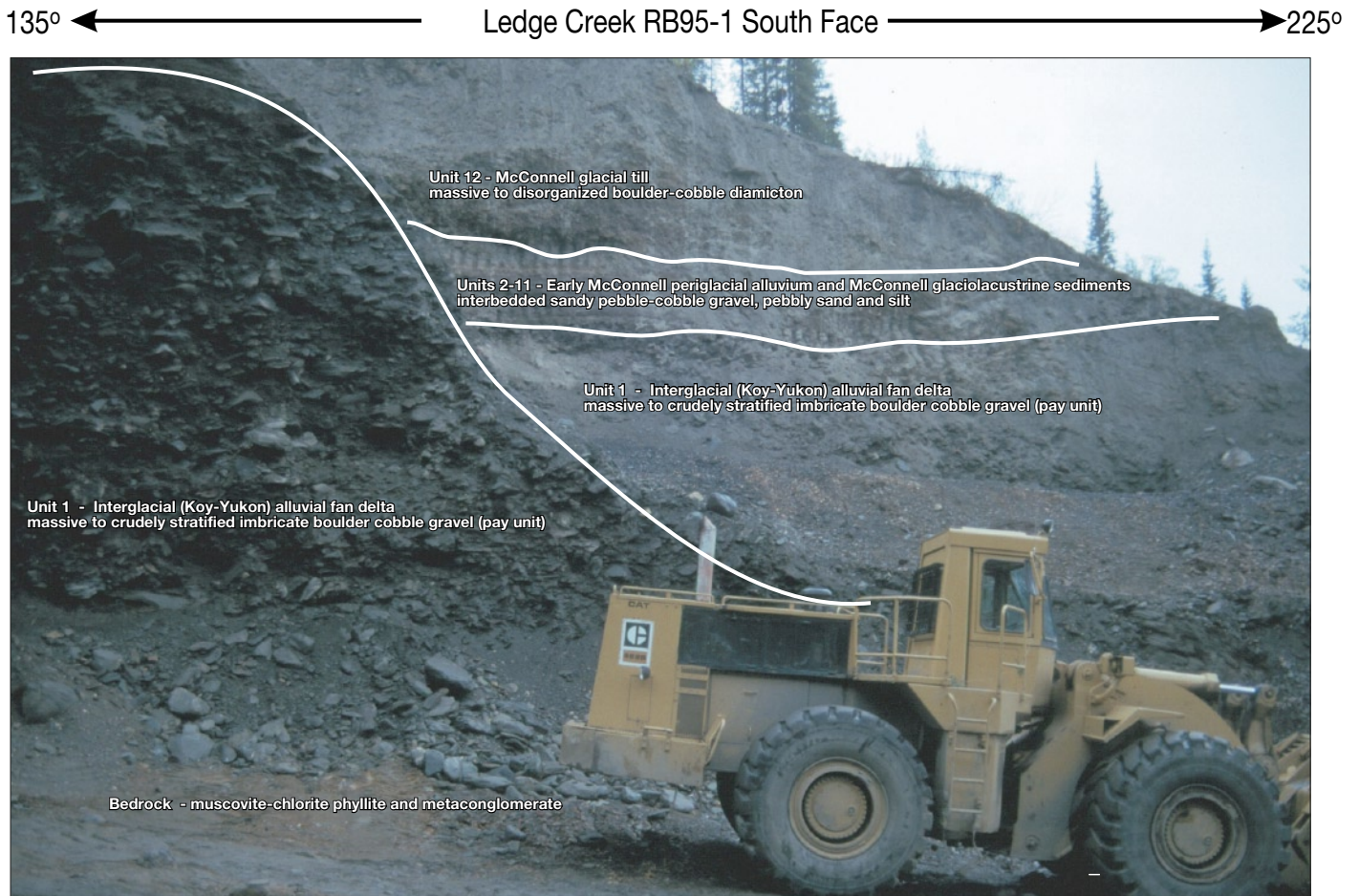
Figure 33. Measured section RB1-95 on Ledge Creek showing interglacial (pre-McConnell) alluvial fan-delta gravel overlain by McConnell glaciolacustrine silt and glacial till. Interglacial gravel is typically gold-bearing, coarse grained and very poorly sorted.
