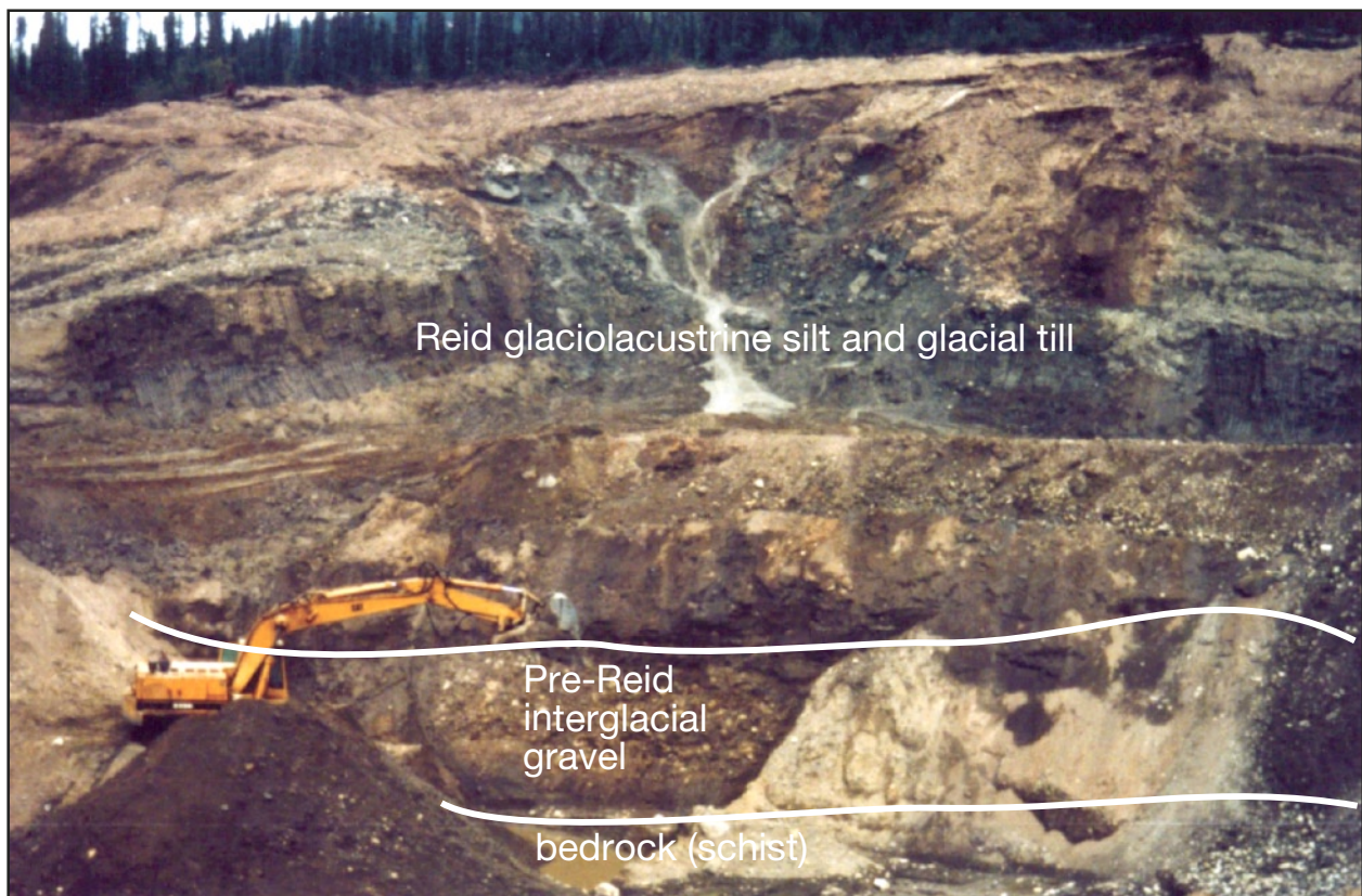
Figure 49. Placer mining in 1995 on the left limit of Haggart Creek exposed gold-bearing pre-Reid interglacial gravels beneath Reid glaciolacustrine silt and glacial till, in measured section RH95-2.
