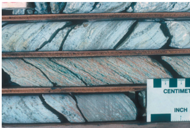
Figure 51. Strongly quartz-carbonate altered Ordovician-Silurian gabbro sill in Grum deposit. Sill is strongly foliated and is located in middle row of core. Drill hole FAGU189, 17.9-25 m. BQ-size core.
