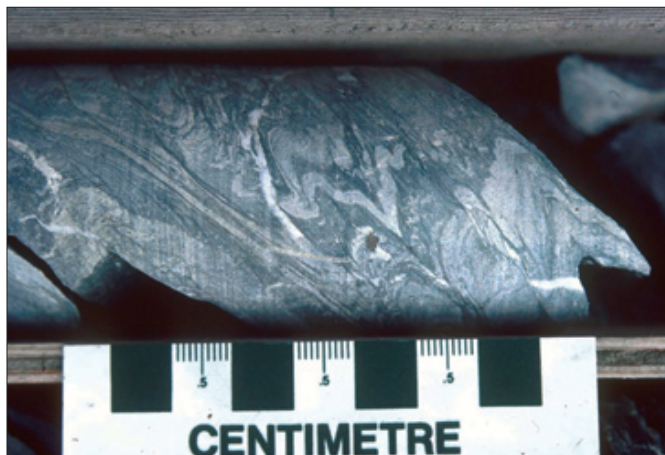
Figure 60. D_1 minor fold defined by siltstone bed in Vangorda formation. Drill hole 76X-11, 72 ft (22 m). Drill hole located in Dy /Grizzly deposit area. NQ-size core.
