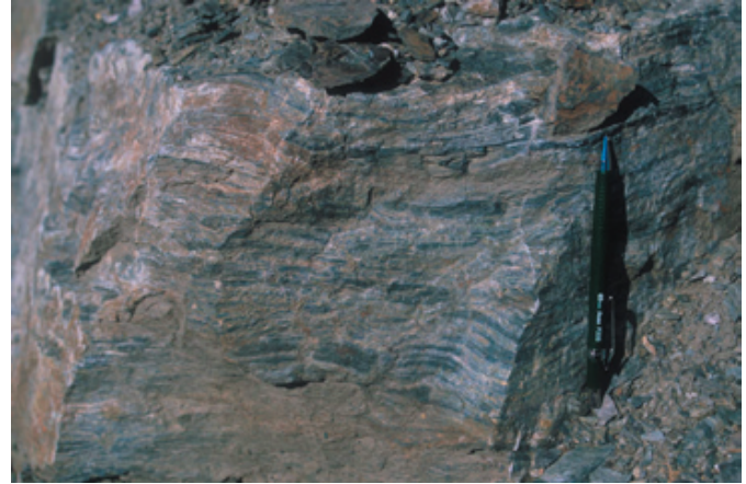
Figure 17. Vangorda formation. Calc-silicate rock outcrop in southwest wall of Faro deposit open pit. Pale green calc-silicate rock bands and lenses, interbedded with dark purplish brown to grey biotite-rich bands and lenses. Pencil on right side of photo is 14.5 cm long.
