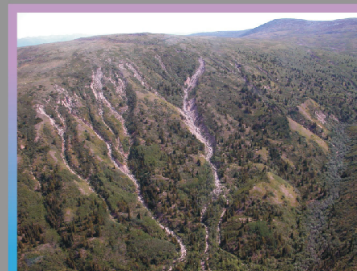
8 Mount Sumanik Oblique aerial view of flow-related debris flows on Mount Sumanik. A 60 cm saturated soil plastic layer was discovered on top of the frozen soil above the initiation zone of the flows.
