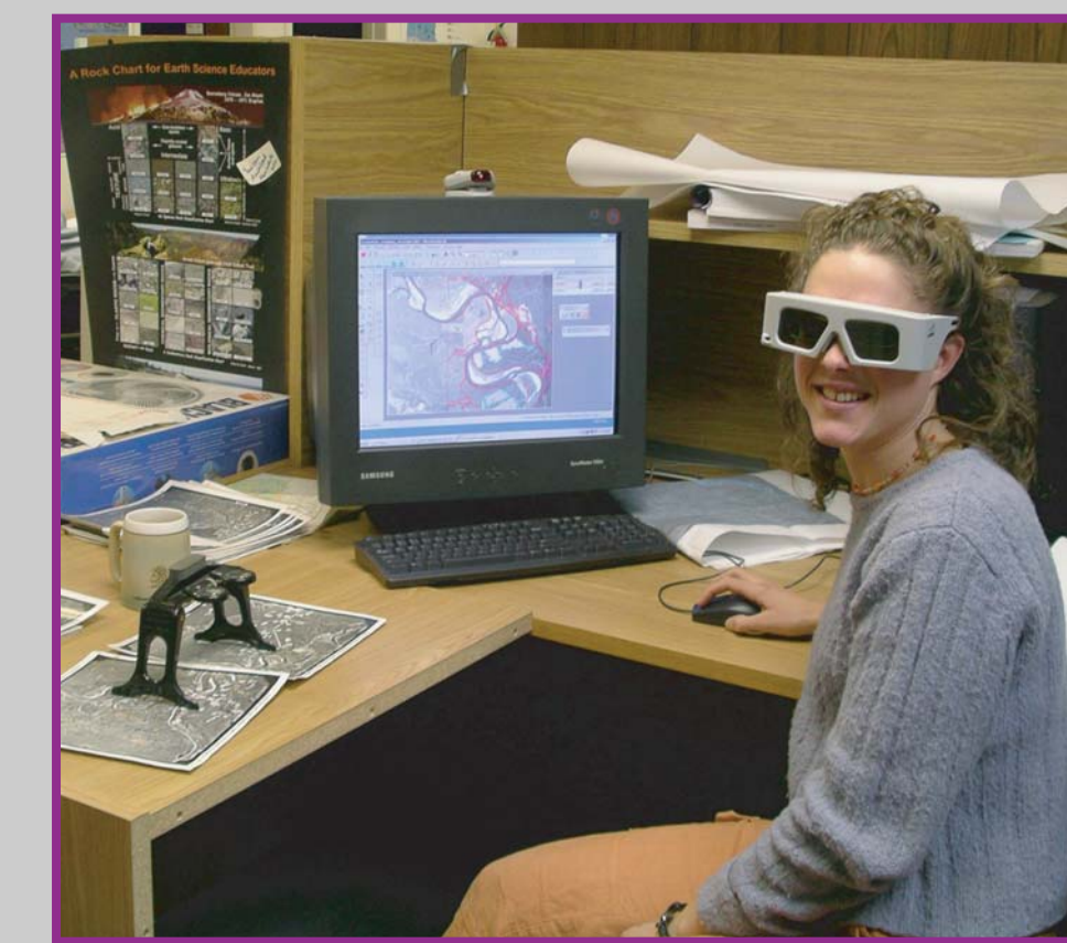
Figure 2. MicroStation DIAP Viewer stereoscopic glasses and work station for digital air photo interpretation.
