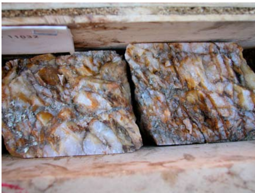
Figure 26. Quartz-pyrite vein mineralization from the Shamrock zone at Ketz River.
