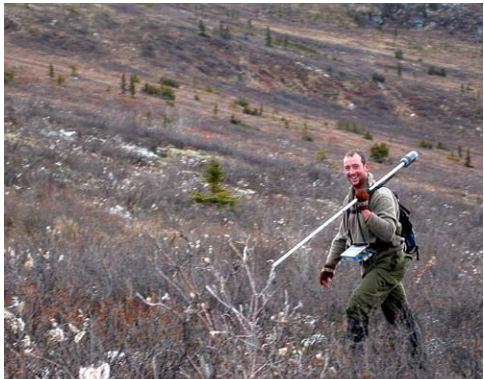
Figure 29. Mike Lindley with Ryanwood Exploration conducting magnetometer surveying on the Blackfox property.
