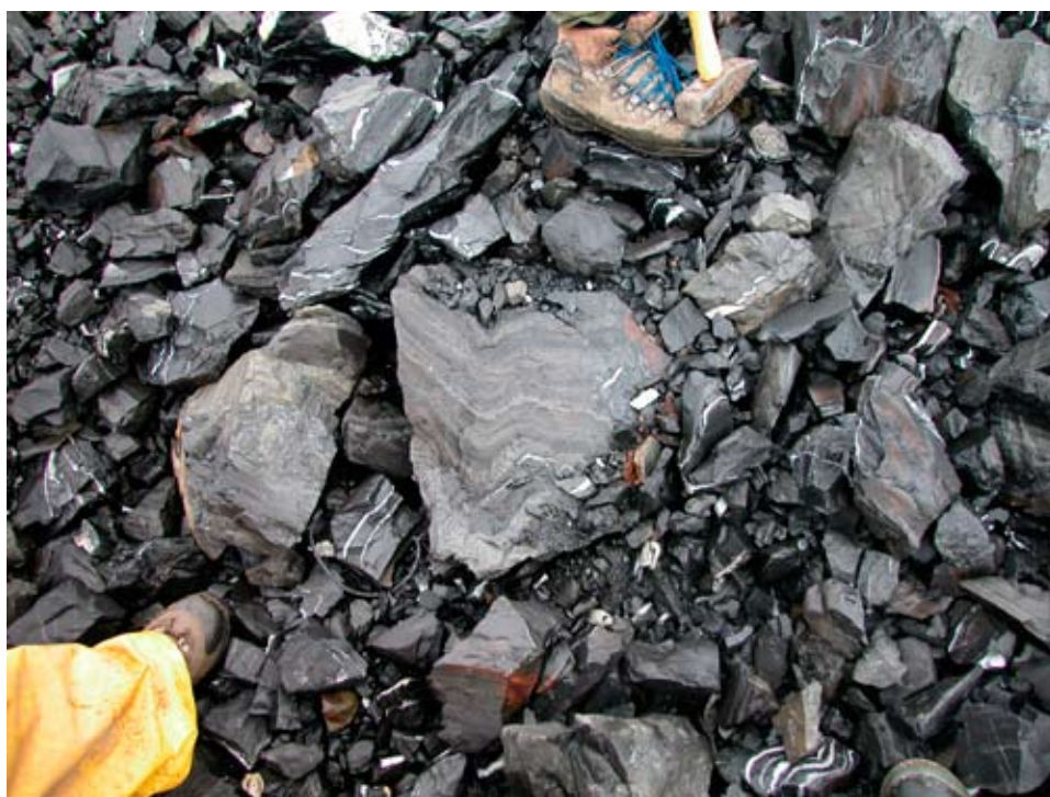
Figure 16. Fine-grained sphalerite, pyrite and galena occur in rhythmically laminated carbonaceous chert and calcareous mudstone at the Howard's Pass deposits.
