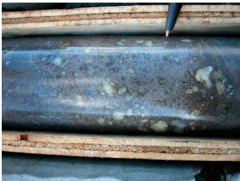
Figure 25. Massive pyrrhotite-pyrite manto-style mineralization from Ketz River.
