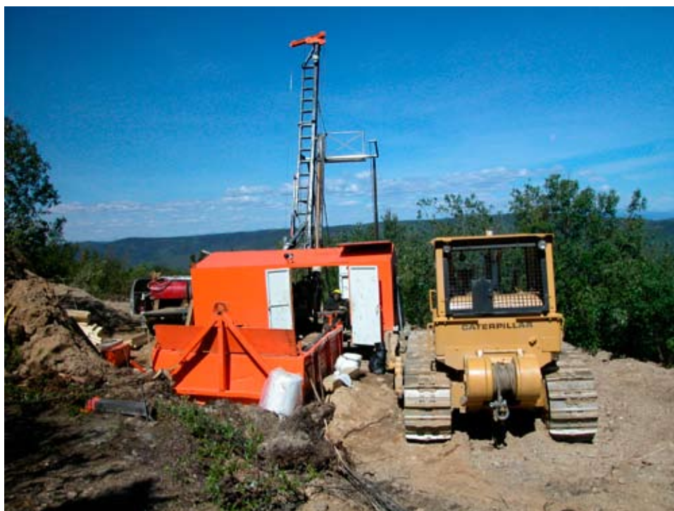
Figure 27. Diamond drill on the Lone Star property.
