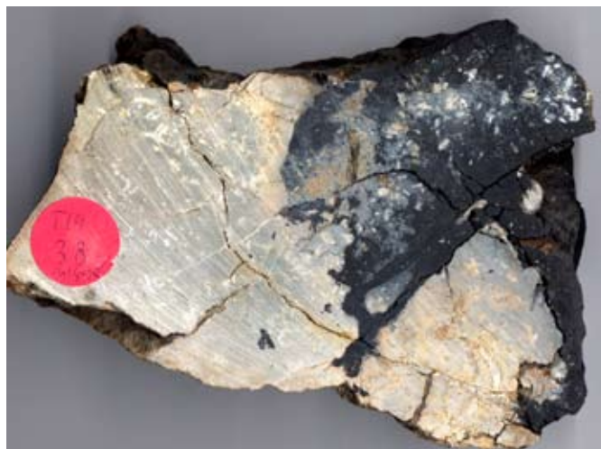
Figure 2. Peperite (white and grey flecks, top right) and natural coke (black) produced by intrusion of a felsic porphyry dyke (left and lower right) into water-saturated medium- to low-volatile bituminous coal, Mount Granger, Whitehorse. Age of the dyke is not known.
