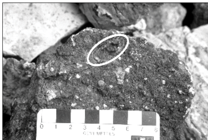
Figure 5. Dark green, ovoid, serpentinized mantle xenolith (circled) from sample 2.
