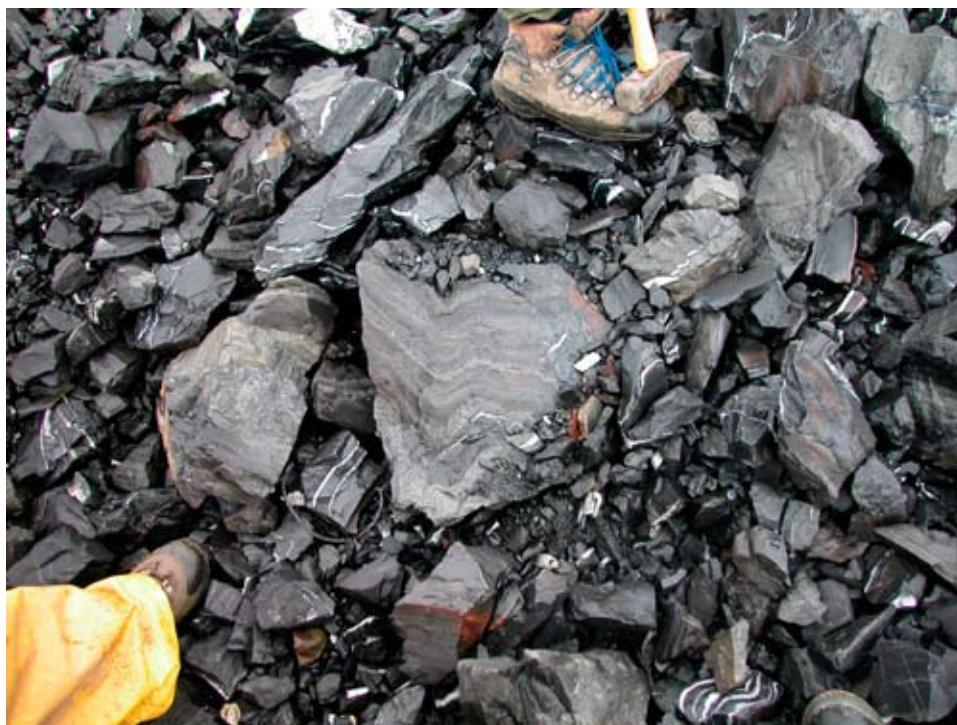
Figure 16. Fine-grained sphalerite, pyrite and galena occur in rhythmically laminated carbonaceous chert and calcareous mudstone at the Howard's Pass deposits.
