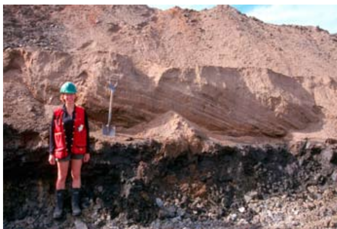
Figure 13. Technogenic deposit, measured section 60M01-03. Typical dredge tailings with planar-tabular-stratified sandy gravel over mud and bedrock. Fractured bedrock here contains economic gold values.
