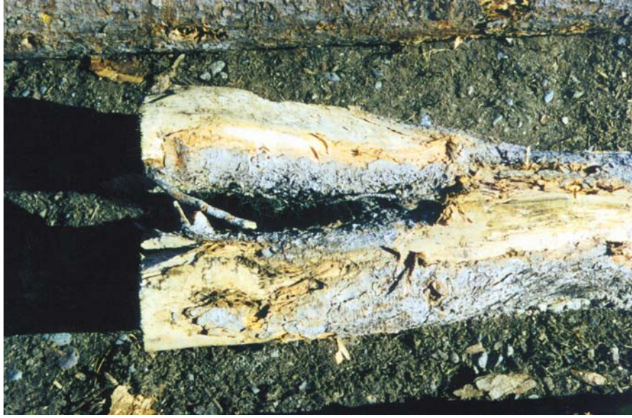
Figure 10.21 This log was bucked above the crotch, with the separate stems cut at an even length
