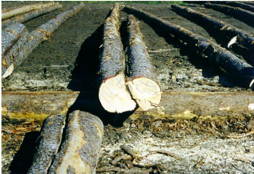
10.22 This log was bucked so the top two stems can be scaled as separate pieces
