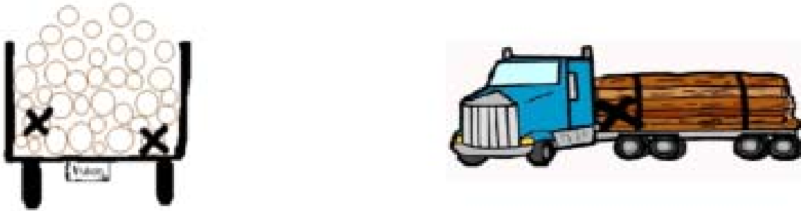
Figure 15.6 Load marking requirements for round wood
