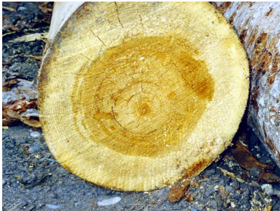
Figure 3.1 Various stages of heart rot
