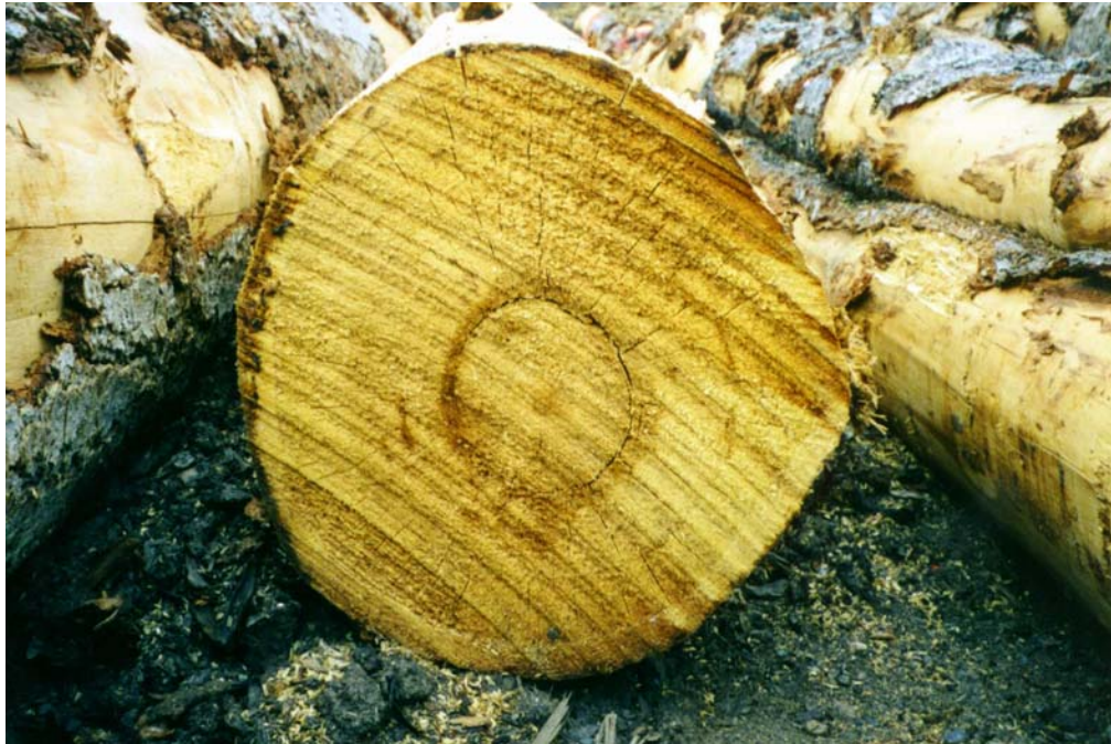
Figure 5.4 Ring rot encompassing 100% of the circumference of the log
