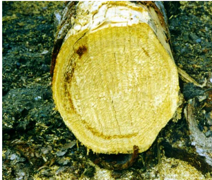
Figure 5.1 Ring rot encompassing approximately 45% of the log circumference
