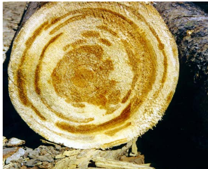
Figure 5.2 Ring rot in various stages on the collar, heart rot in the centre
